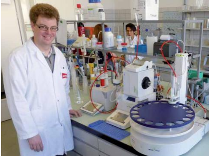
Figure 1: Mr. Kunz, the Quality Assurance Manager at RAMSEIER Suisse AG, and the measurement system comprising an InMotion™ Flex Autosampler, DM40 density meter, RX50 refractive index cell, and T90 titrator.
